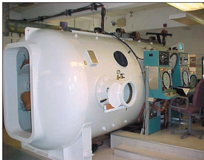
Fig. 1: Eight-person hyperbaric chamber. One or more patients are monitored by inside attendant(s) and observed through a window and on video. Communication between patients and the outside chamber takes place by intercom. There is a small portal for passing medicines, food and other necessities. Usual treatment lasts 286 minutes.
